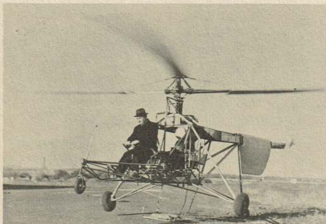
The Sikorsky VS-300 with Mr. Sikorsky at the controls.
